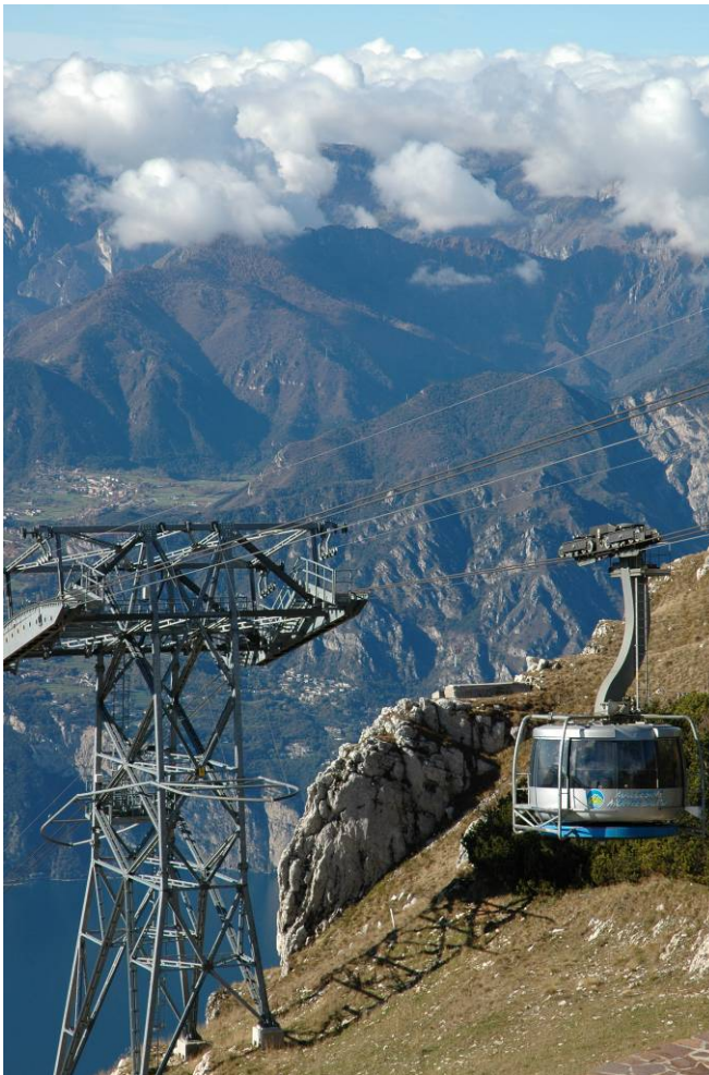
Car with revolving cabin with 80 person capacity
